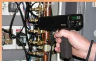
Detect air leaks
