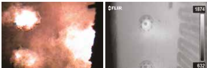
Some FLIR thermal imaging cameras can measure the temperatures behind the flames.
