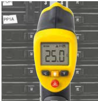
IR thermometer, temperature measurement in one spot
