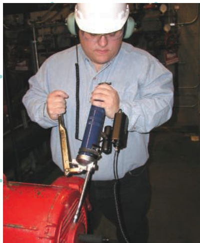
Listen while applying grease
