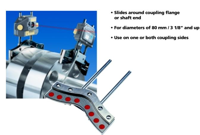
Shafts can't be rotated? No problem! This bracket allows measurement and alignment to be performed when one or both shafts cannot be rotated. The magnetic sliding bracket is placed upon the back of the coupling or front corner of the uncoupled shaft and slid around from one measurement position to the next. Suitable for shaft/coupling diameters from approx. 80 mm (3 1/8") on up.
