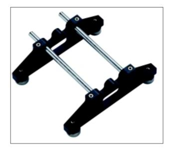
This bracket can replace the compact chain-type bracket for large couplings having correspondingly large bolt holes. Especially handy when radial clearance around the coupling rim is limited, this bracket allows the laser beam to be directed through a coupling bolt hole with the emitter and receiver mounted below the rim.
