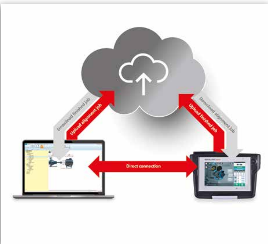
Real-time communication between ALIGNMENT RELIABILITY CENTER 4.0 and ROTALIGN® touch via the Cloud
