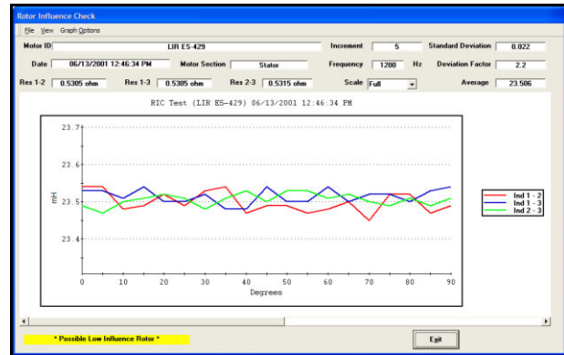
Figure 19. Inductance Test of a Rotor With “Low Influence”
