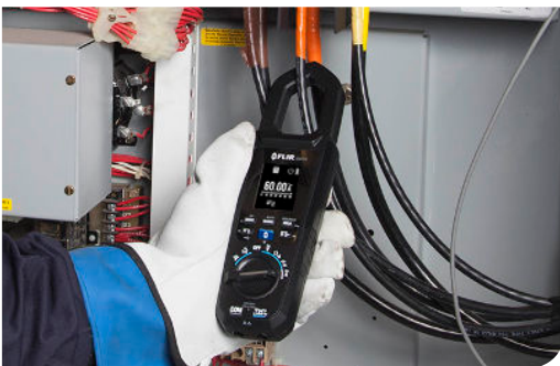
Verify amperage measurements
