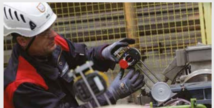
Laser-optical alignment of an installed cardan shaft
