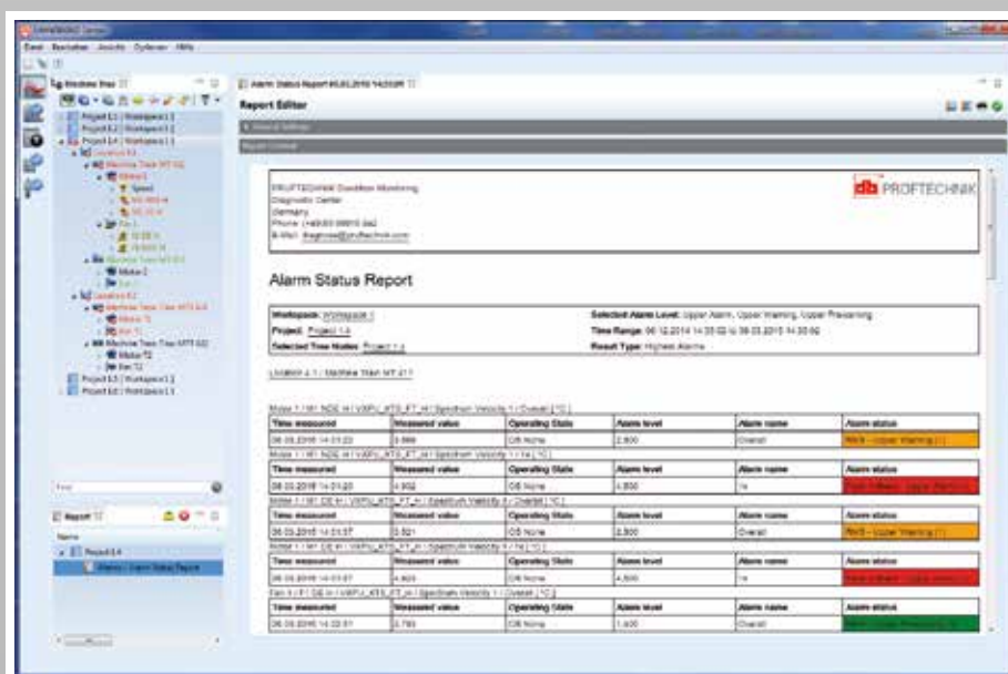
Alarm status report displays critical machine conditions
