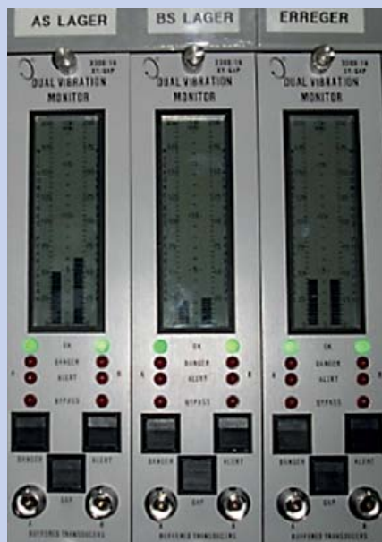
Fig. 7: Measuring device for shaft vibrations; special water pump and mounted balancing weights
