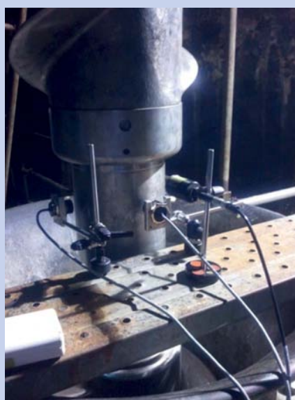
Fig. 11: Balancing of a mixer on the basis of orbit measurements
