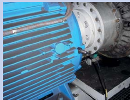
Fig. 8: Conveyor drive motor with accelerometer; hydraulic clutch with washers as balancing weights
