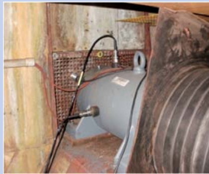
Fig. 6: Induced draft, measurement locations on the bearings and FFT spectra before and after balancing
