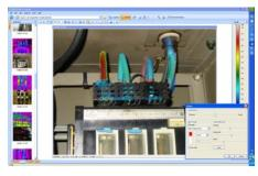
Analyzing in Fusion view - blend IR image and corresponding visual image together using Image Fusion technology, making interpretation of your work even easier
