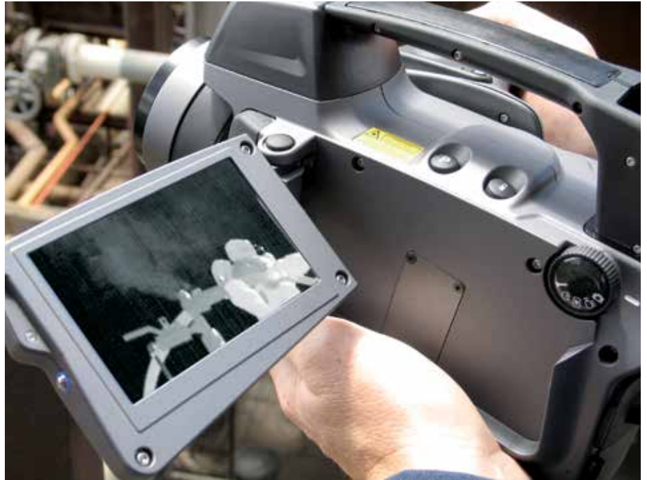
Optical gas imaging cameras allow you to detect even small leaks from a safe distance.
