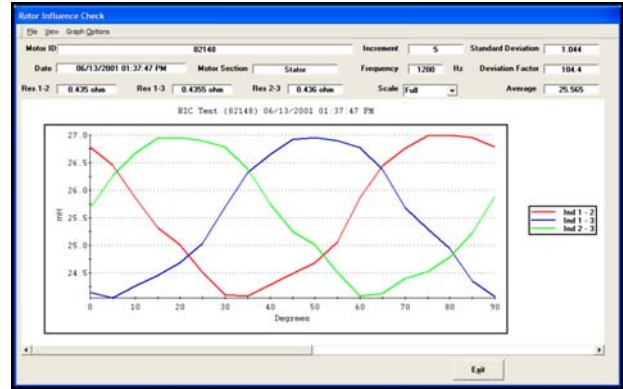
Figure 13. Repeated Variations Throughout All Three Phases of Inductance
