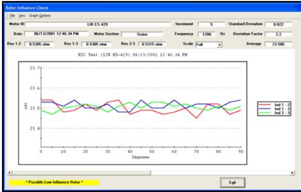
Figure 11. Inductance Test of a Rotor With “Low Influence”
