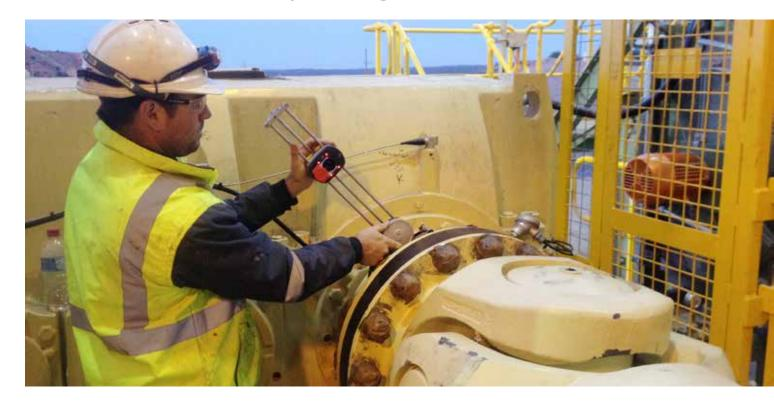
LSmidth is a global engineering company supplying one source plants, systems and services to the cement and minerals industries. In September 2013, the company needed to perform the alignment of a three-machine train with two cardan shafts at a gold mine in Western Australia. The machine train consisted of an arrangement of conveyor pulley, gearbox and motor.
