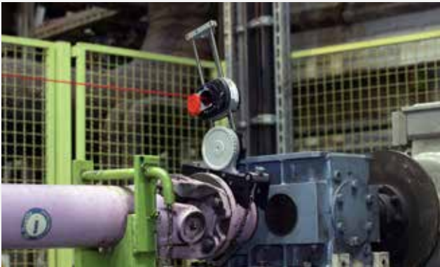
Rotating arm bracket for restricted rotation areas.
