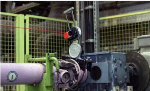
Rotating arm bracket for restricted rotation areas.
