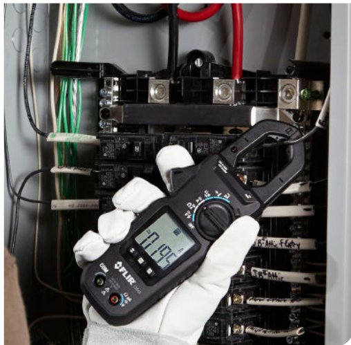
Accu-Tip enables more accurate amperage measurements
